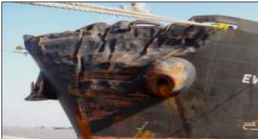
Figure 10: Damages to the bow, anchor and anchor chain
